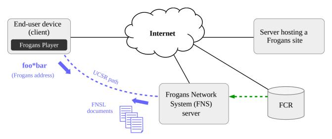
Figure 3. Resolution of a Frogans address via an FNS server
