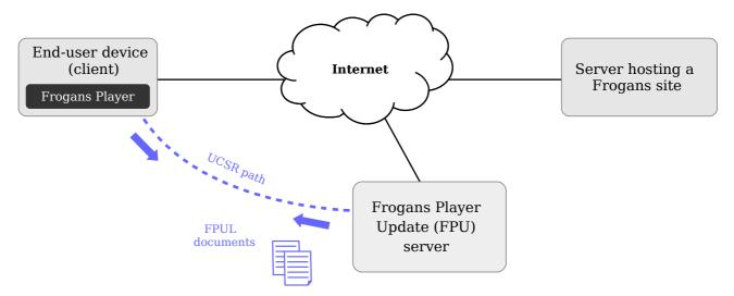
Figure 5. Checking if Frogans Player is up to date via an FPU server
